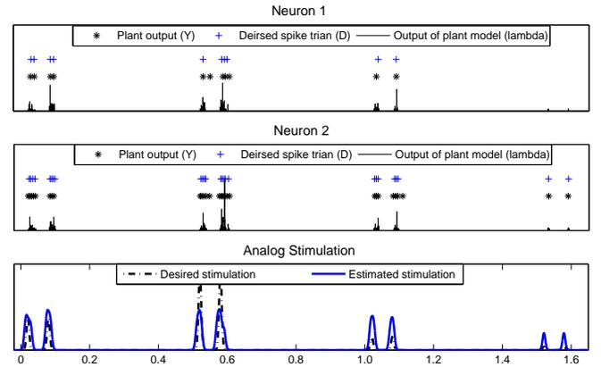
Fig. 5. The tracking performance of the MIMO adaptive controller. The first two plots show the target spike trains (D), the output of the plant (Y), and the plant model output ( $\lambda$ ) of the output neuron O1 and O2, respectively. The bottom plot compares the estimated stimulation that elicit the output spike train and the desired stimulation that elicit the target spike train.
