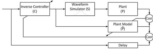
Fig. 1. The adaptive inverse control system diagram
